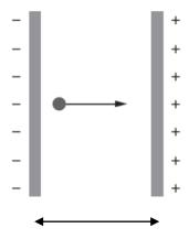
A proton is launched from the negative plate with speed u. The proton just reaches the positive plate and instantaneously stops before turning back.
