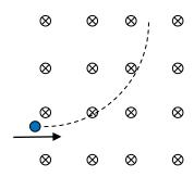
The proton exits the region of magnetic field after completing a quarter of a circle.
